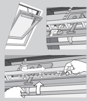
In case of power failure or discharged battery, your centre-pivot window can be closed manually by disengaging the chain on the ventilation flap of the window.
