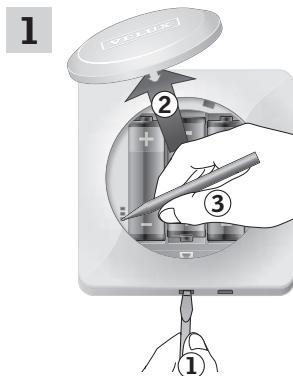
Remove the battery compartment lid by pressing the release button with a screwdriver as illustrated ①, ②.
