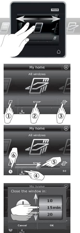
You operate all products by tapping icons/buttons or by dragging the slider and tapping the bar in the display.
